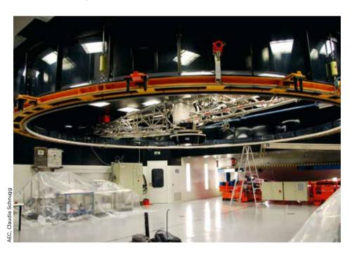
Since the reflector's reflective coating deteriorates over time—due to oxidation or wear and tear—these sensitive elements have to be recoated every few years.
