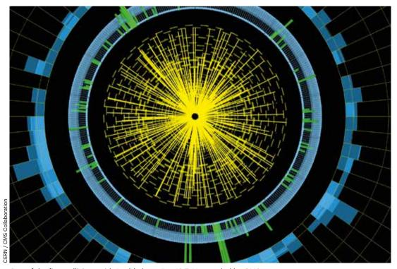
One of the first collisions with "stable beam" at 13 TeV recorded by CMS.
