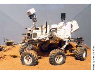
Open Curiosity is an open source ExoMars rover (1:5 scale) that facilitates affordable space exploration for all. Based on the NASA Curiosity Rover, it uses Arduino. Data gathered (temperature, pressure, radiation, distance, wheel position, arm position) is available on the internet for educational, scientific, or other purposes. Sensors detect obstacles to avoid collisions and it has a HD video camera.
