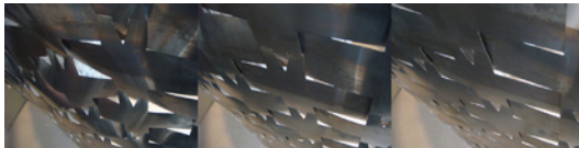
Fig. 1: Thermobimetal automatically curls when hot (left) and flattens when cold (right).
