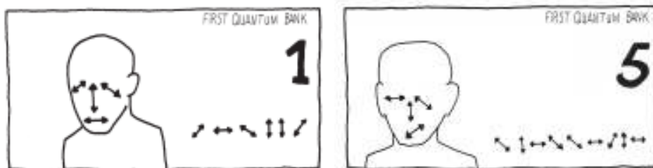
Figure 1: Unforgeable quantum money. A number unique to each quantum bill is printed using quantum bits ( qubits ). Since quanta cannot be cloned, such quantum money cannot be forged. Actually, the specific state of the qubit, indicated by the double arrows, is only shown for illustration. It cannot be seen directly, and it cannot be measured directly unless one already knows what the number is. This information would be restricted to the national bank printing the money.
